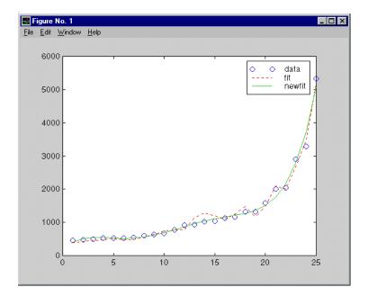
Since the data is closely correlated but not exactly linearly dependent, the fit curve (dashed line) shows a close, but not an exact, fit. The fifth-degree polynomial curve, newfit, represents a more accurate mathematical model for the data.
